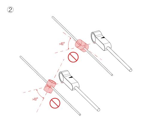
3. Check whether the speed measuring magnet is aligned with the " $\triangle$ " mark of the speed sensor.
